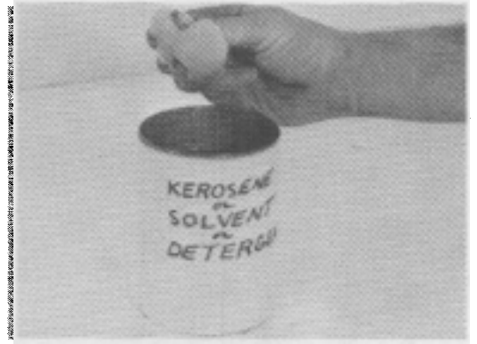
Fig. 35—Wash filter in kerosene, petroleum solvent or detergent.
