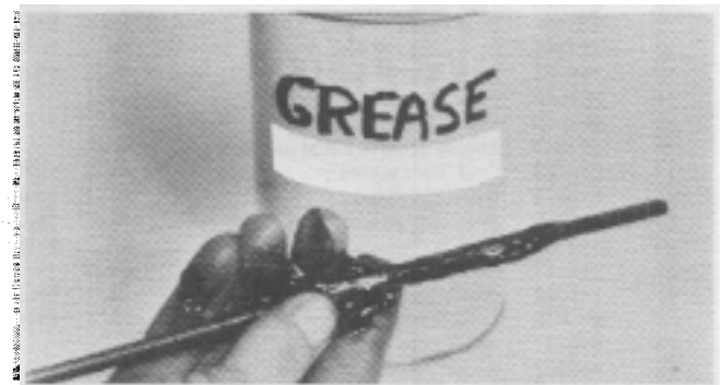
Fig. 39—IMPORTANT: Anytime flexible drive shaft core is removed from outer housing, it should be cleaned and regreased with high speed, high temperature wheel bearing grease, Mobil #532 or equivalent.
