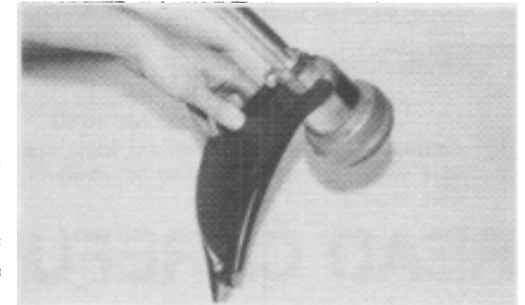
Fig. 9—Drop guard down to top of aluminum bearing housing and rotate guard into proper position.
