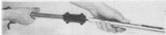
Fig. 4—Insert loose end of Flex Drive Shaft into upper portion of Trimmer Boom. It may be necessary to rotate Cutting Head Assembly to be sure Flex Shaft is properly engaged into engine portion of Trimmer Boom.
