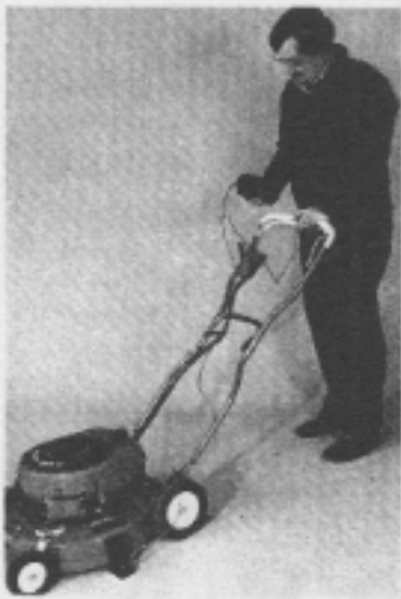
ET-301 Mower Monitor on compliant mower checking blade stoppage time.
