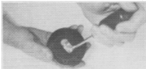
Fig. 7—To replace reed if necessary, remove two mounting screws as shown.
