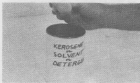
Fig. 3 — Wash filter in kerosene, petroleum solvent or detergent.
