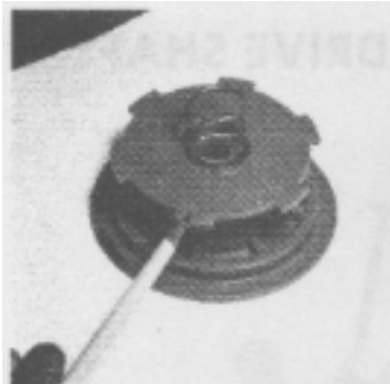
Fig. 37 — Check indexing teeth on inner and outer spool for wear. If necessary, replace.
