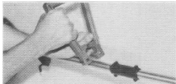
Fig. 7—Remove "D" handle from package. Spread and twist "D" handle enough to interlock tabs as it is being installed over tube. Install bolt, washer and wing nut and tighten.
