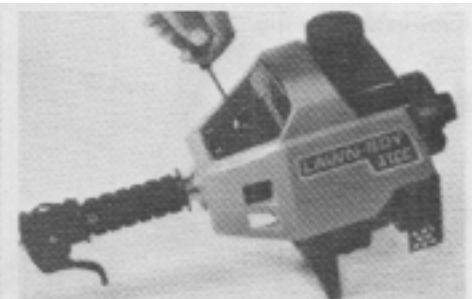
Fig. 15—Operator with unit in starting attitude. Depress the throttle trigger and pull starter rope in a brisk manner with the unit in the above position.
