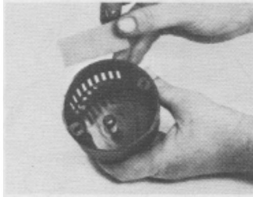
Fig. 34—Remove filter from carburetor cover.
