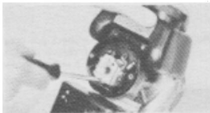
Fig. 2—Remove carburetor mounting screws.
