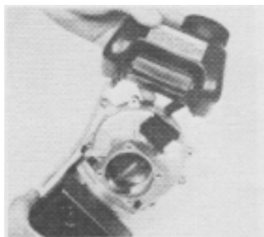
Fig. 10—View showing tank removed from shroud assembly. Also at this time check condition of tank for any rubbing or chaffing spots. Replace if necessary.
