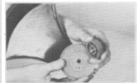
Fig. 34—Hold outer spool with one hand and unscrew bump knob in counterclockwise direction. Inspect bump knob to be sure it can freely move axially on the captured bolt.
