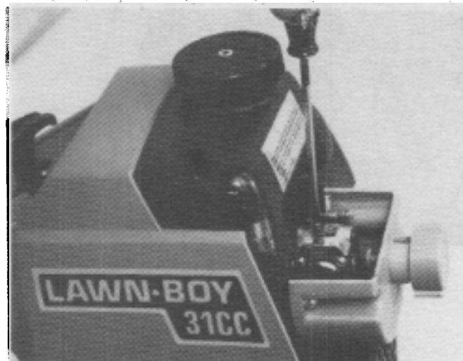
Fig. 18—View showing low speed mixture carburetor adjustment.
