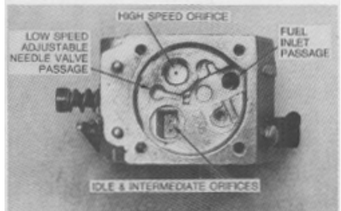
Fig. 18—Correct procedure to clean this carburetor is wash in solvent and blow all passages with compressed air.
