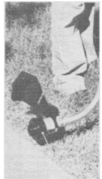
Fig. 25—When edging, let the top of the trimming line do the work. Cut with trimmer in the position shown.
