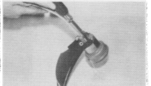
Fig. 11—Tighten all four guard screws before running unit.
