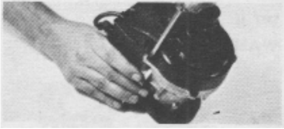
Fig. 1—Remove four mounting screws from starter housing.
